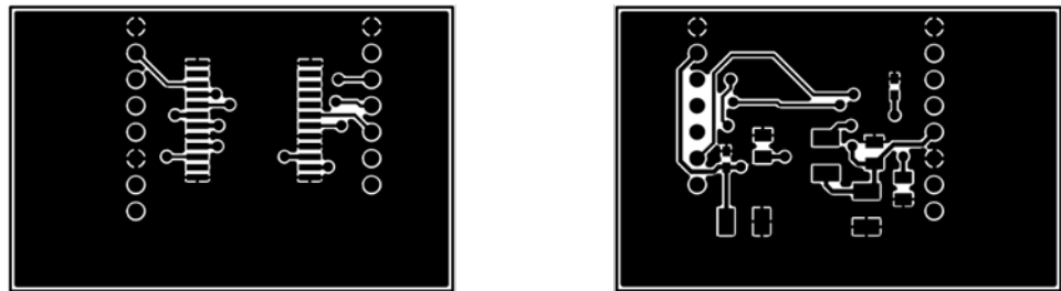
Figure 2. TOP (left) and BOTTOM (right) layout of SCC2000 series PCB (aspect ratio not 1:1).
