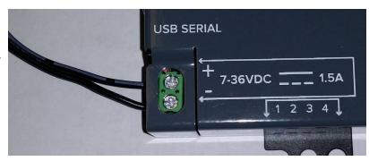
when connecting power to the E12, don't worry because the input is reverse polarity protected.
