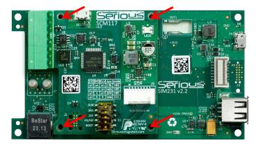
Using four machine screws gently fasten the SCM117 into the SIM's standoffs. These M3-0.50 screws should be no more than 6mm in length.
