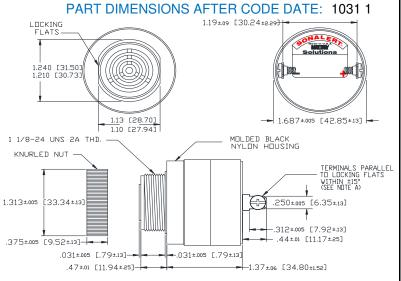
NOTE A: TERMINALS-.032 BRASS TIN PLATED, TAPPED FOR #6-32 SCREW, TVO #6-32 NICKEL PLATED BRASS SCREVS INCLUDED, WILL ACCEPT 1/4' QUICK CINNECT. NOTE B: MOUNTING- REMOVE BLACK PLASTIC NUT AND INSERT THREADED FRONT THROUGH 1.25' HOLE PUNCHED IN PANEL, IF DRIENTATION IS NEEDED, NOTE LOCKING FLATS ON DRAWING, SCREW NUT BACK ON. DO NOT OVERTIGHTEN.
