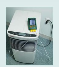
Simultaneously record and time stamp multiple temperature readings.
