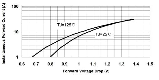
Fig.3-Typical Instantaneous Forward Voltage Characteristics
