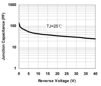
**Fig.1-Typical Junction Capacitance**
