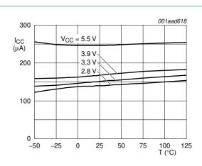
Fig 13. Typical normal I<sup>2</sup>C-bus inactive supply current as a function of temperature
