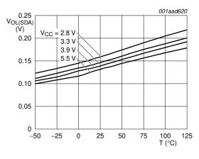
Fig 15. Typical SDA V<sub>OL</sub> as a function of temperature
