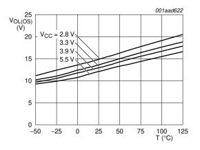
Fig 17. Typical OS  $V_{\text{OL}}$  as a function of temperature
