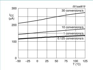
Fig 14. Typical normal I<sup>2</sup>C-bus inactive supply current as a function of temperature
