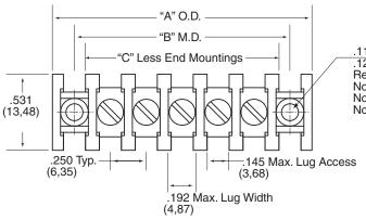
.116 Dia. Hole Both Ends Recommended MTG Screws No. 2 BD. or PAN HD No. 3 MAX RD HD
