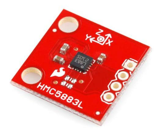
**Triple Axis Magnetometer Breakout - HMC5883L**
