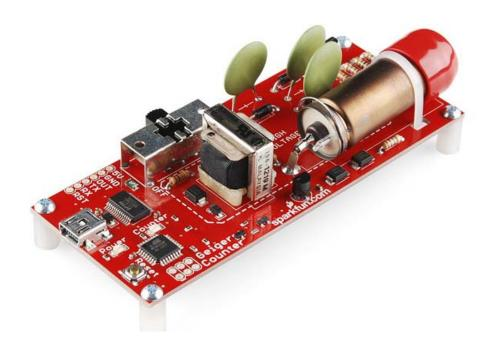
**Description:** You talked, we listened, and we've revised our Geiger Counter board to address some of the most pressing concerns. This version features an improved voltage regulation circuit for the Geiger tube which has a much cleaner output. We've also modified the signal capture portion of the board so that it reads active high, allowing for more dependable counts that are less susceptible to fouling due to line capacitance. The new signal capture circuit also pushes the CPM limit to 100Hz!
