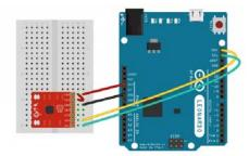
Here's everything all hooked up. Make sure you add the small jumper from VDD to VIO to ensure they are both connected to 3.3V.
