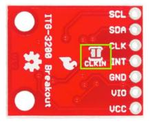
Make sure you close this jumper with solder if you're NOT using an external clock source.
