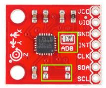
Here the I<sup>2</sup>C address jumper (top) and the unpopulated I<sup>2</sup>C pull-up resistors (bottom) are highlighted.
