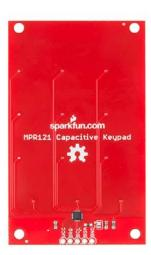
**Description:** The MPR121 capacitive keypad uses the MPR121 and 12 touch sensitive pads to give you a simple 'keypad' with an I<sup>2</sup>C output. These keypads function by measuring the capacitance of twelve electrode points. When an object comes close to the electrode connector, the measured capacitance changes. This signals the MPR121 that something has touched a 'button'.
