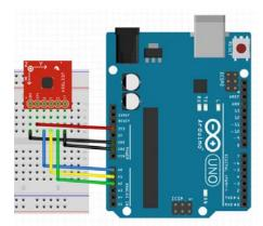
We simply have to supply the accelerometer with power (3.3V and GND), then hookup the X, Y, and Z lines of the sensor to ADC pins (A0, A1, and A2 respectively in this case). The self test pin (ST) can be left disconnected or connected to ground under normal operation. If you want to use the self test to double check the functionality of the sensor, tie it to 3.3V. Check the datasheet for more info.
