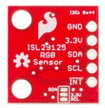
If you want to disable the on-board 10k $\Omega$  I<sup>2</sup>C pullup resistors – in case you want to use those built into your microcontroller or other external pull-ups – simply cut the two traces between the three pads on the backside of the board. If you decide you want the pull-ups later, you can always solder the pads back together.
