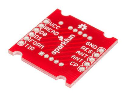
**Description:** This is a simple breakout board for our RFID readers. The SparkFun RFID Reader Breakout converts the 2mm pins to bread board friendly 0.1" headers. With this ability the ID-3LA, ID-12LA, and the ID-20LA you can solder the reader directly to the breakout board or use the 2mm sockets.
