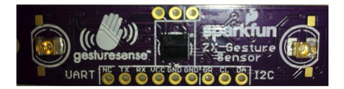
Note the labeled connections are shown here— it is important that the FTDI cable goes is connected to the UART portion of the pin-out. I2C connections are for only the 3 pins on the right, as well as using VCC and GND connections to power the sensor.
