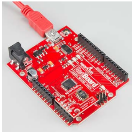
A SHT15 connected to a SparkFun RedBoard, using pins A4 and A5 as communication and pins A2 and A3 as power.
