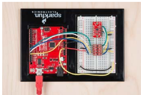
The circuit built on a RedBoard
