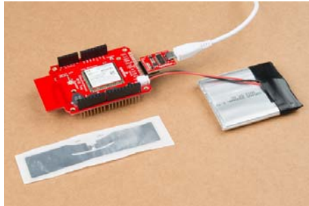
LiPo Battery powering the RFID shield
