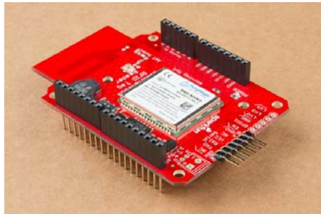
Shield with stackable headers installed.
