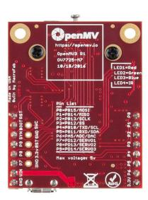
**Description:** The OpenMV M7 Camera is a small, low-power microcontroller board that allows you to easily implement applications using machine vision in the real world. The best part about the OpenMV is that it is not only capable of image capture, but also face detection, color tracking, QR code reading and plenty more. If you are looking for an economical camera module boasting multiple high-end features, look no further than the OpenMV M7!
