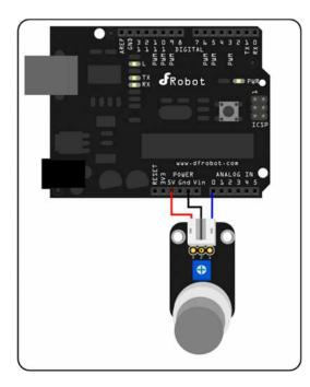
Analog sensor connection diagram
