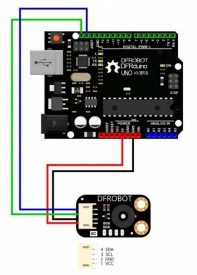
IR Thermometer Sensor-MLX90614 Wire Diagram
