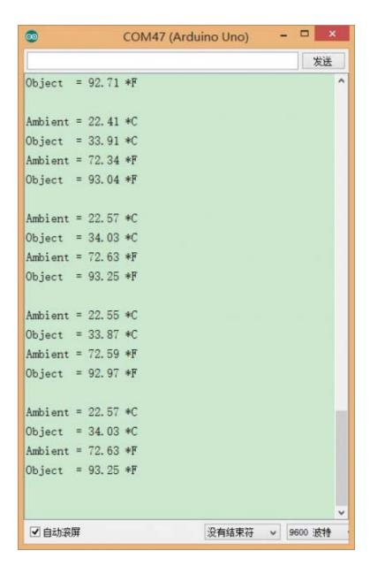
IR Thermometer Sensor-MLX90614 Test Result
