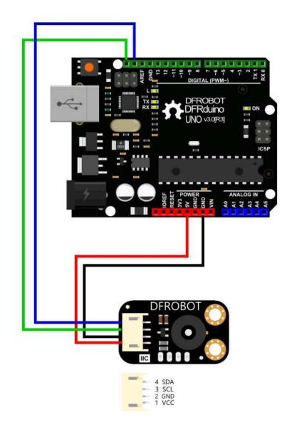
SEN0263 (MLX90614-DCI), due to its small field of view (FOV = 5°), is more suitable for industrial applications where the detection distance can be longer. In general applications, you can use SEN0206(MLX90614-BCC)
