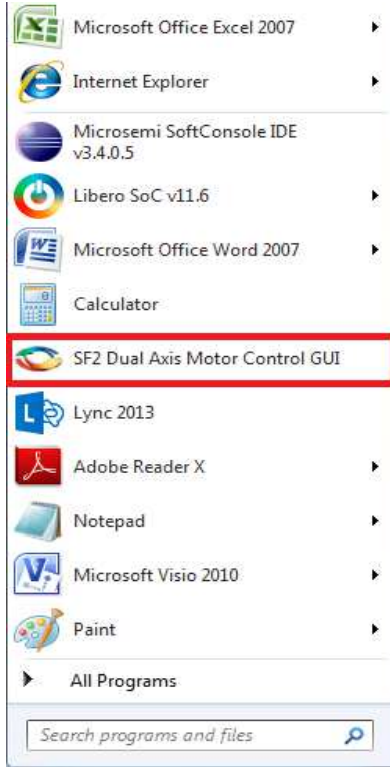
Figure 13 • Launching the SmartFusion2 Dual-Axis Motor Control GUI
