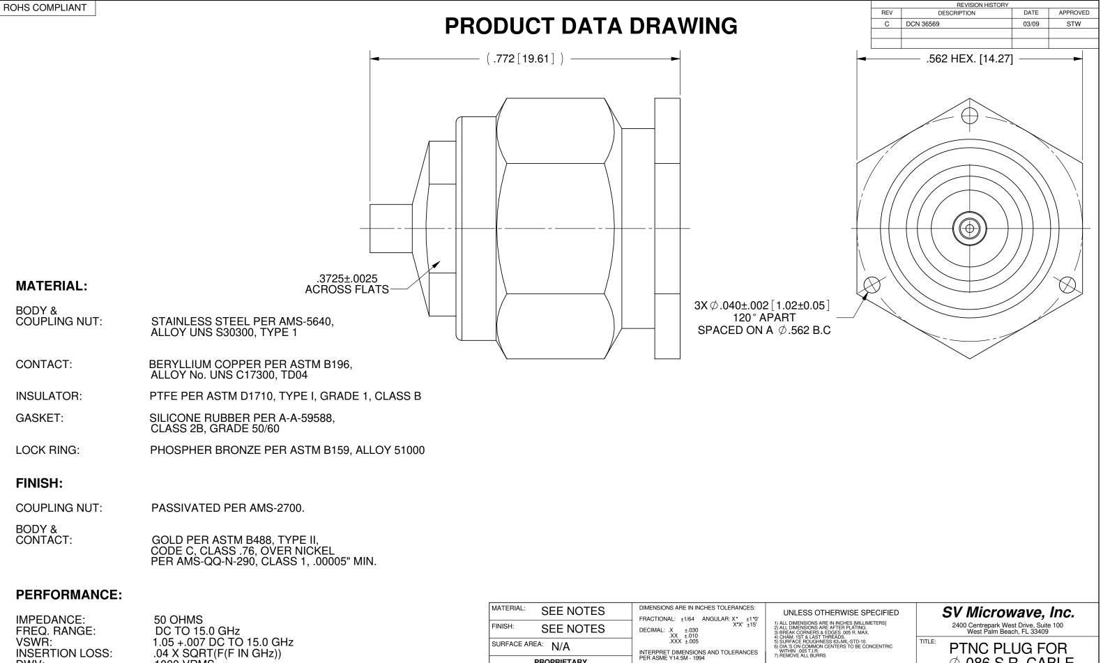
**INSERTION LOSS:** DWV: **INSUL. RES.: OPERATING TEMP:**  .04 X SQRT(F(F IN GHz)) 1000 VRMS 5000 MEGOHMS. -65° TO +165°C
