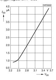
Current consumption  $I_{DD}$  in ALS mode  $I_{DD} = f(V_{DD})$ ; Register 0x41= 0x08
