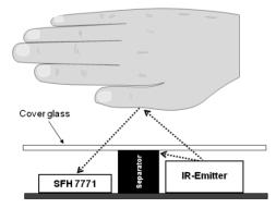
When proximity sensing is performed, it is desirable that only light from a reflecting object reaches the SFH 7771. Depending on the optical setup, additional and unintended light paths from the IR-Emitter to the detector may exist, which is referred to as '(optical) crosstalk'. One measure to avoid such crosstalk is to add a separator between emitter and detector as drafted in the picture below. For details please refer to our SFH 7771 application note.
