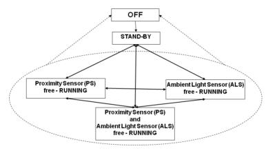
If  $V_{DD}$  exceeds the threshold voltage, the sensor will switch from OFF mode to STAND-BY mode. As shown in the transition-diagram above it is possible to switch between all modes without any restriction.
