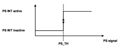
**01 PS\_TH & PS\_TL (PS high & low threshold) are active as hysteresis:** PS\_TH and PS\_TL are working as a hysteresis. If the PS measurement signal is higher than the PS high threshold (PS TH) the INT state is switched to active. If the PS measurement signal is lower than the PS low threshold (PS TL) the INT state is inactive. If once interrupt signal becomes active, INT status is kept active until measurement result becomes less than PS TL reqister value.
