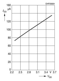
Current consumption I<sub>DD</sub> in PS mode
