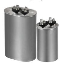
Type SF, AC rated metallized polypropylene capacitors provide starting torque and power factor correction for split phase motors typically used in refrigeration and air conditioning motor-run applications. Type SF also may be used to provide noise suppression, voltage regulation and line current reduction in power supply applications.
