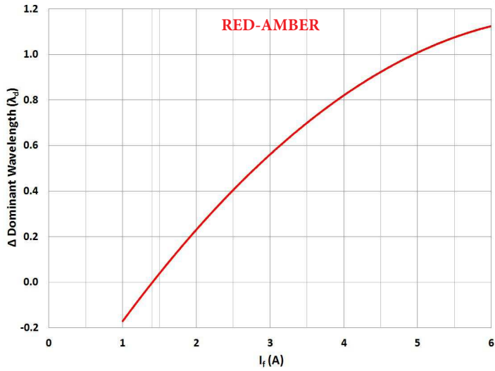
vs. Forward Current ( T_{hs} = 25^{\circ}\text{C} , I_f = \text{Pulse} )
