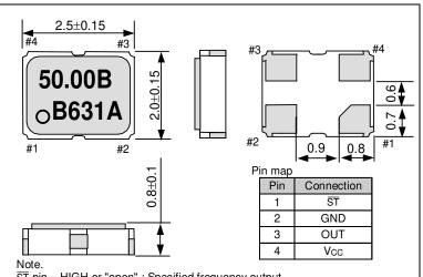
ST pin = HIGH or "open" : Specified frequency output.
