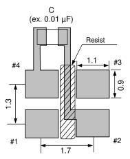
To maintain stable operation, provide a 0.01uF to 0.1uF by-pass capacitor at a location as near as possible to the power source terminal of the crystal product (between Vcc - GND).
