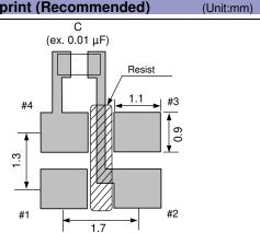
To maintain stable operation, provide a 0.01 $\mu$ F to 0.1 $\mu$ F by-pass capacitor at a location as near as possible to the power source terminal of the crystal product (between Vcc - GND).
