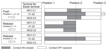
3 position enabling switch: 2 contacts; pin No.: NO1-C1, NO2-C2 Push monitor switch: 0, 1 contacts: pin No.: 31-32 (SG-C1-21)
