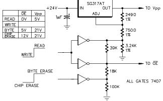
Figure 24 – 2816 EEPROM Supply Programmer for Read / Write Control
