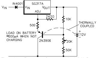
**Figure 25** – Temperature Compensated Lead Acid Battery Charger
