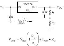
Figure 17 - Basic Regulator Circuit
