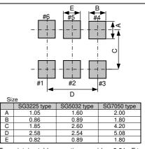
To maintain stable operation, provide a 0.01 µF to 0.1  $\mu$ F by-pass capacitor at a location as near as possible to the power source terminal of the crystal product (between Vcc - GND).
