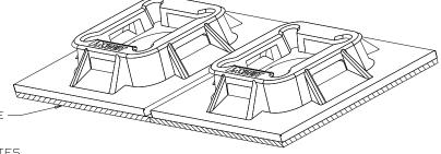
ADHESIVE BACKING: (-A , -AT) RUBBER OR ACRYLIC BASED ADHESIVE PRESSURE SENSITIVE FOAM TAPE 0.04 [1.0] THICK WITH A PROTECTIVE LINER. MOUNT IS DESIGNED TO SUPPORT 0.50 lbs (227g) MAX. WEIGHT ON A CLEAN DRY SMOOTH SURFACE.
