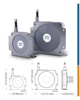
Suited for IP67 (wet) environments, the SGD provides a user-selectable 4-20mA or 0-10VDC absolute linear position signal over an 80-inch or 120-inch full stroke range option. Signal selection is simply made by connecting the appropriate pins on the included connector or selecting the proper wires in the optional cordset.
