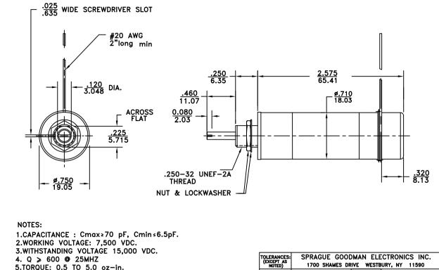
6.OPERATION TEMPERATURE: BELOW -55°C UP TO 125°C 7.DIMENSIONS IN INCHES/MM. 8.ROTATIONAL LIFE: 10.000 TURNS 9.CONSTRUCTION: SEALED, NON MAGNETIC
