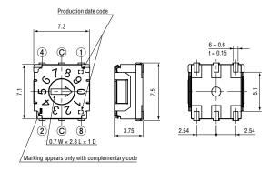
Unless otherwise specified, tolerance:  $\pm$  0.3 (Unit: mm)
