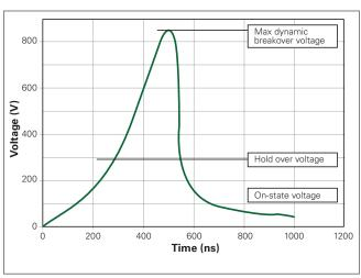
Note: Tested per 1kV/µs waveform
