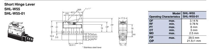
Note: Unless otherwise specified, a tolerance of  $\pm 0.4$  mm applies to all dimensions.
