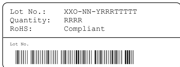
Figure 20: First label on reel: XX = Sensor Type (20 for SHT20), O = Output mode (D = Digital, P = PWM, S = SDM), NN = product revision no., Y = last digit of year, RRR = number of sensors on reel divided by 10 (200 for 2000 units), TTTT = Traceability Code.
