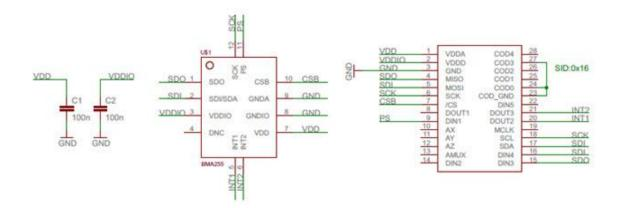
BMA253 shuttle board electrical layout
