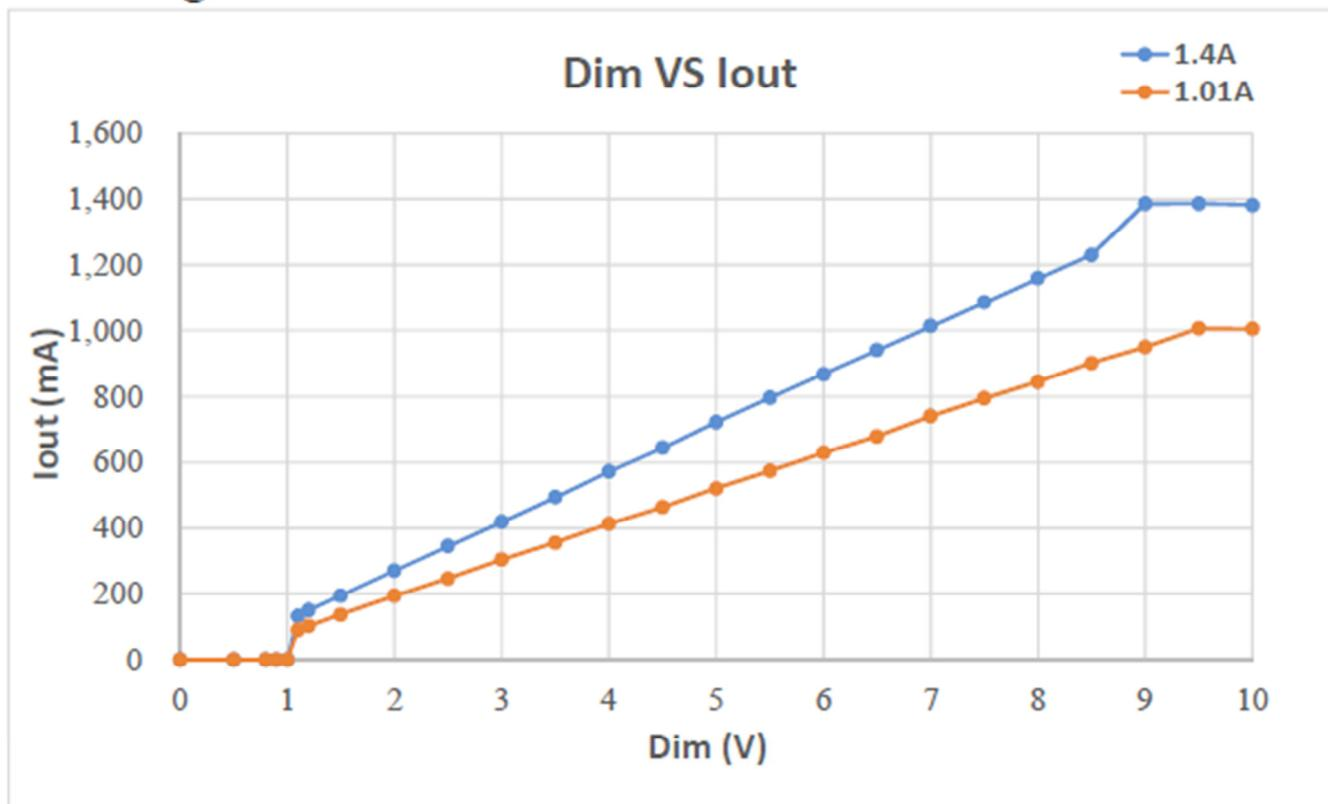
Note: The dimming curve is tested with LED electronic load Chroma 63115A/6312A. Rd coefficient is 0.16.
