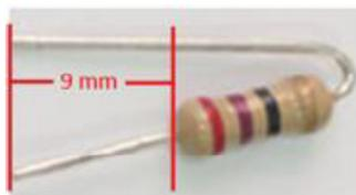
Insert the resistor to the Rset connector
