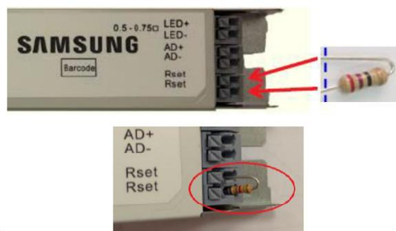
※ Resistor wire should be the opposite side of driver metal case.
