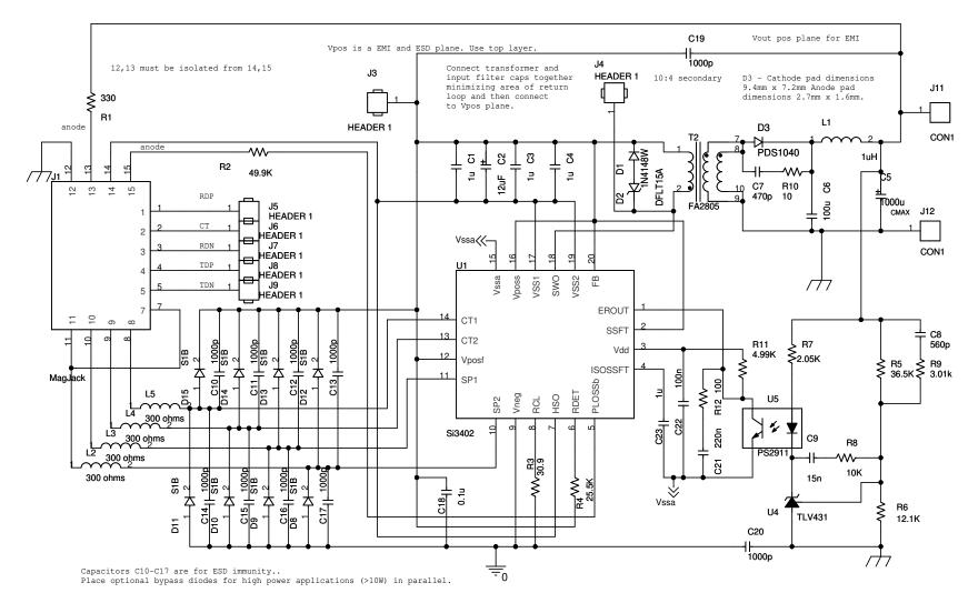
Vneg is a thermal plane as well as ESD and EMI. Use thermal vias to at least 1 inch square plane on backside 1 to 1.2mm pitch 0.3 to 0.33mm diameter.
