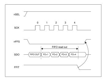
During FIFO access  $f_{\text{SCK}}$  cannot be higher than  $f_{\text{ref}}/4$ , where  $f_{\text{ref}}$  is the crystal oscillator frequency.
