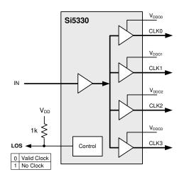
Figure 2. LOS Indicator with External Pull-Up
