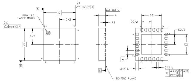
Figure 4. 24-Lead Quad Flat No-Lead (QFN)
