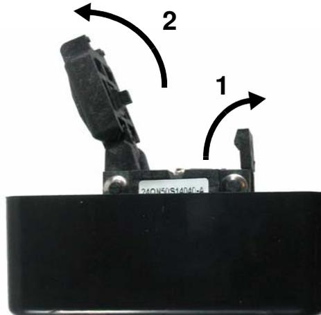
2. Insert a blank Si5338 or Si5356 device in the socket using a pair of tweezers or a suction tool. **It is very important that the Si5338 or Si5356 be inserted into the socket with the correct pin 1 orientation.** Pin 1 on the device is marked with a white dot. Pin 1 on the socket is labeled on the PCB as shown below.
