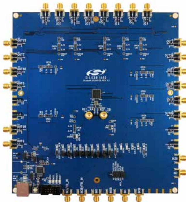
Figure 1. Si5345-D Evaluation Board
