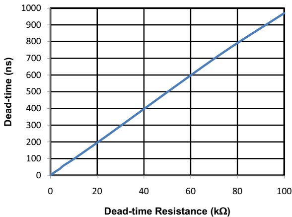
Figure 37. Dead Time vs. Resistance ( R_{DT} )
