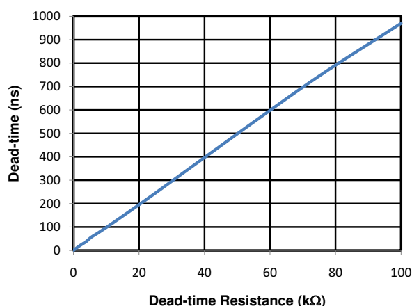
Figure 37. Dead Time vs. Resistance ( R_{DT} )
