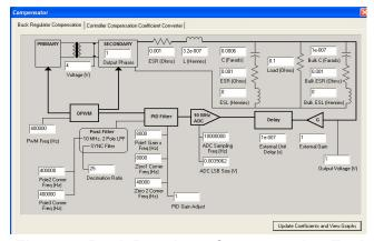
Figure 5. Buck Regulator Compensation Tool
