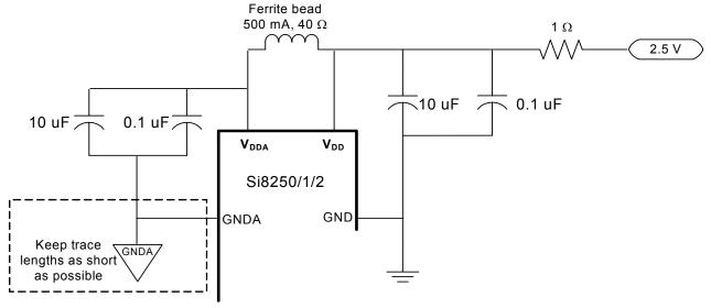
Figure 10. Power Supply Connections for LQFP-32 Package
