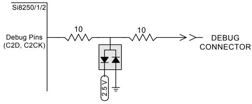
Figure 12. Debug Interface Pin Protection Circuit
