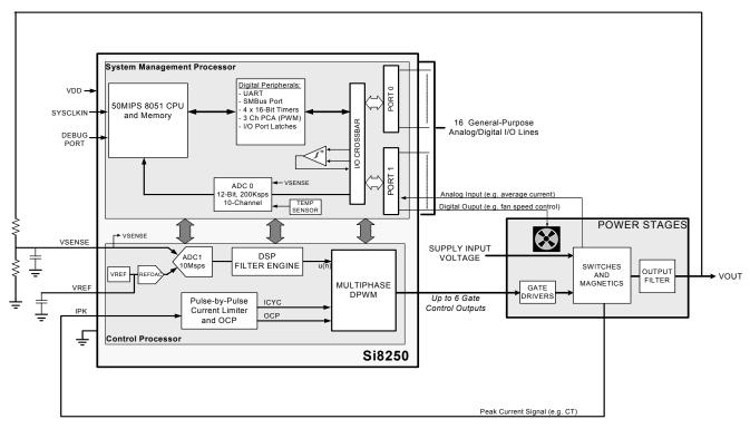
Figure 2. Si8250 Top-Level Block Diagram
