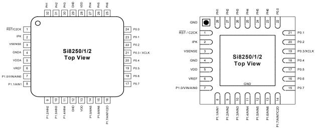
Figure 13. Example Pin Configurations
