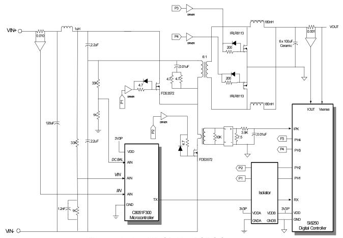
Figure 7. Isolated Half-Bridge DC/DC Converter
