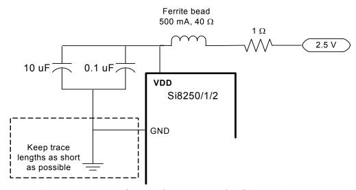
Figure 11. Power Supply Connections for QFN-28 Package
